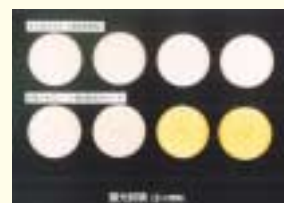
Light stability test of cosmetics raw materials The Vaseline Shiseido uses has fewer impurities than the usual Vaseline, and is stable under strong light for a long period, not changing in color.
