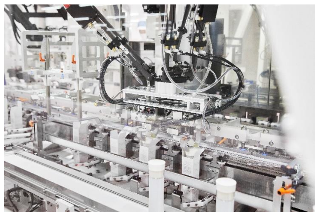
“linear motor-driven cartoner”
